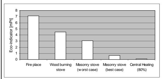
Figure 8.4 Environmental load of the use phase in Eco-indicator millipoints per unit heat produced.
